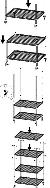
STEP 3. Fit **SHELF (D)** over the top of the 4 poles and over SLIP SLEEVES (E).
