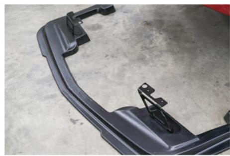
STEP 8: Install brackets - Using the center punch or scribe, mark the holes for the brackets to attach to the radiator support panel of the car. The large hole on the bracket aligns with the large hole in the radiator support as shown. Drill these marks with the 1/8" drill bit, run each screw into the hole once before attempting to install the bracket so that the screws go in easily while you're working overhead holding the bracket.
