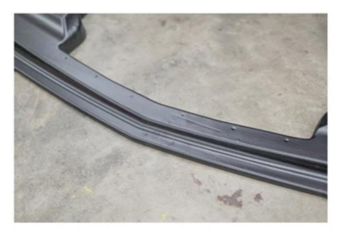
STEP 7: Prep for brackets - Lay out the mounting brackets as shown. Align with holes making sure the brackets are pointing inwards and the vertical section is towards the front of the car. Use the 3/8" drill bit for the six holes for each bracket.
