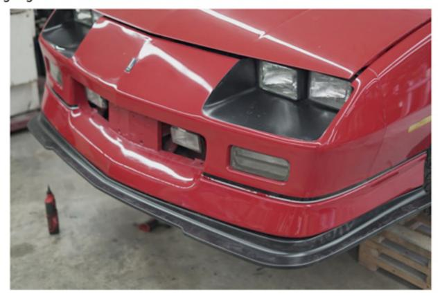
STEP 10: Prepping the corners - Once you are happy with how it roughly sits, it is now time to hand align each corner and mark where the hole will need to be drilled for the factory bolt. Use the 7/16" drill and drill your holes. After aligning both sides, tighten the factory bolt up.
