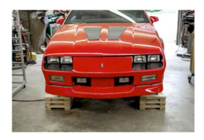
STEP 4: Remove Factory Hardware - This kit is designed to use the 8 holes underneath the factory spoiler extension. 6 are located in the middle front section and one on each rear corner at the fender to body brace. Be sure to remove the plastic clip next to each of the rear holes.
