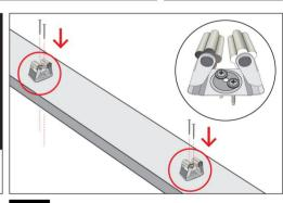
PLACE THE HOLDERS AT THE BOTTOM OF THE WINDOW FRAME.
