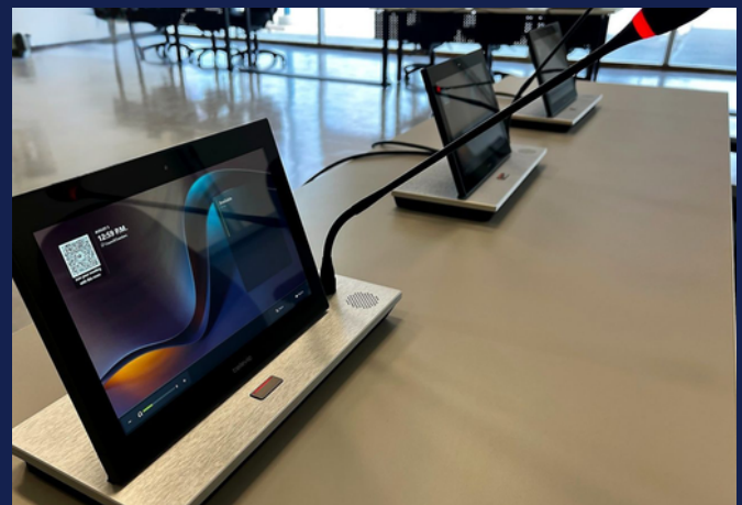
Close-up of the Televic uniCOS multimedia unit with integrated touchscreen and microphone.
