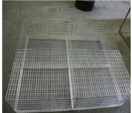
6. This completes a 4'x5' cage section. For a 10' long unit repeat this process and join two sections together, making a 10' long section. Remember the two 5'
