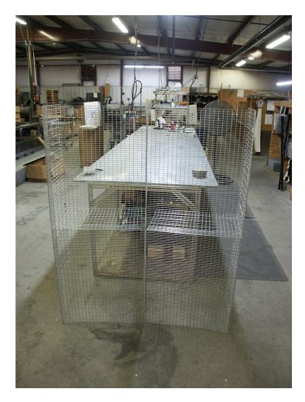
4. You can now clip the 24"x48" 1"x2" wire ends on. Clip 3" intervals on floor and 4" intervals on sides/corners.
