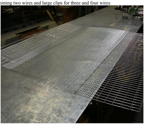
2. Clip wire dividers (1"x2" wire 16"x24"pcs) in center of floor, 30" in from each end. Swing all sides and dividers upward and clip where divider meets the front and back panel in 4" intervals.
