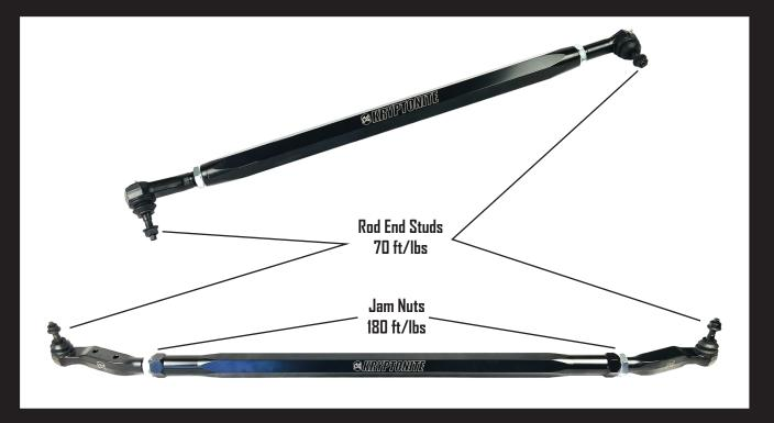
Our drag link is compatible on trucks with up to a 6" lift with the stock pitman arm in use.
