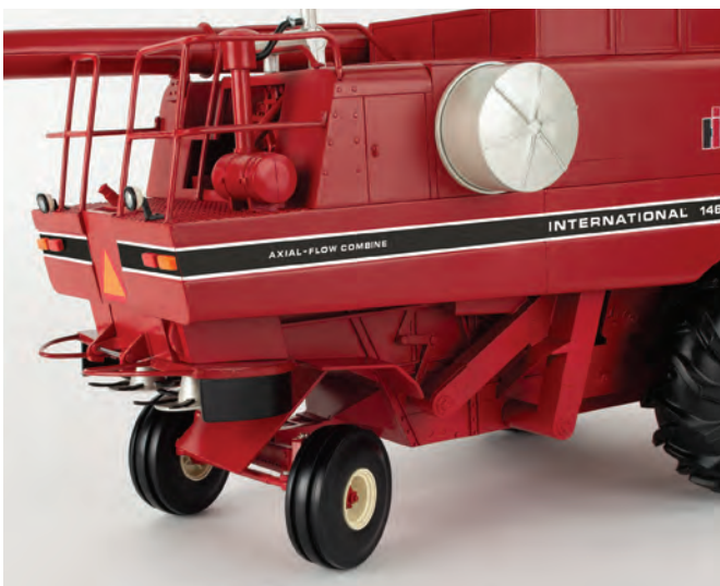
Pivoting rear axle and rotating fan
