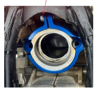
2. Install the M6x1.0x40 . Using an 8 mm socket, tighten the bolts back into place. Make sure they are tightened securely, but don't overtighten them.
