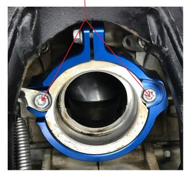
3.Using an 8 mm wrench finish tighten the M6x1.0x12
