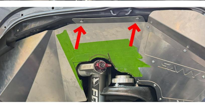
On the driver's side, trim the plastic box shown in the diagram below to allow proper clearance for the inner fender.
