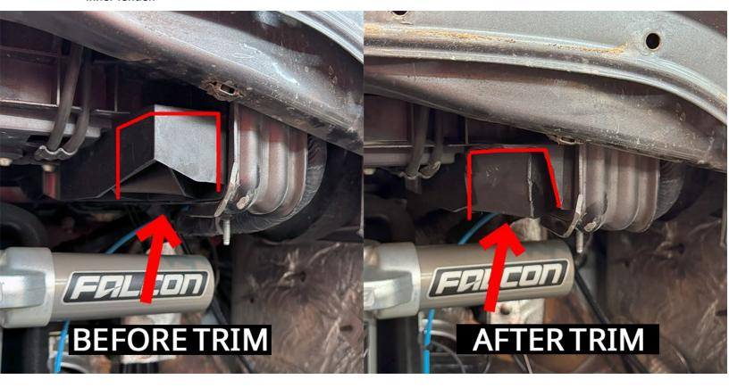
On some Jeep JKs especially if you're running reservoir shocks or need the inner fender to sit further back you may need to trim or grind the areas shown in the diagram below. We've seen some Jeeps clear these brackets with no issue, and others that required minor adjustments. Fitment can vary, so double-check clearance before final installation.
