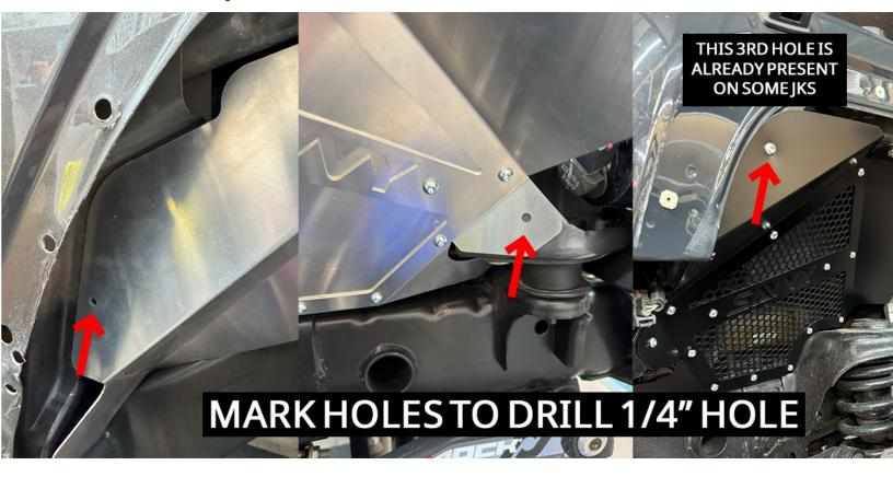
STEP 2: Remove The Inner Fender and Drill 1/4" Holes
