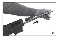
8) Grasp bolt carrier rail to slide the bolt and carrier out of the receiver. The bolt and carrier will separate and you can remove the recoil spring.
