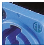
Locking area on chassis connector
