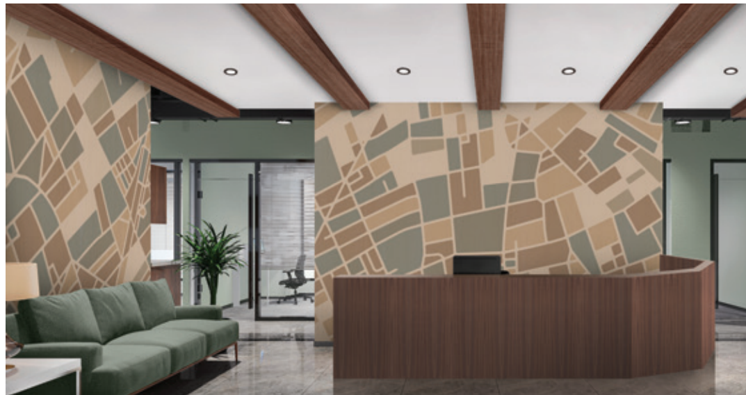
Beams are created with a high-resolution image of Walnut - Quarter Cut wood, printed on Nexa fabric, and wrapped around strips of acoustical panels fabricated into false beams.
