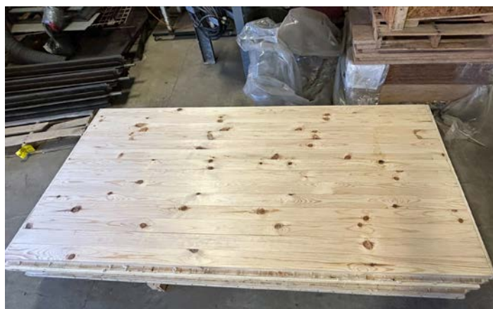
Red pine CLT panel manufactured for Limerick Forest warming cabin.
